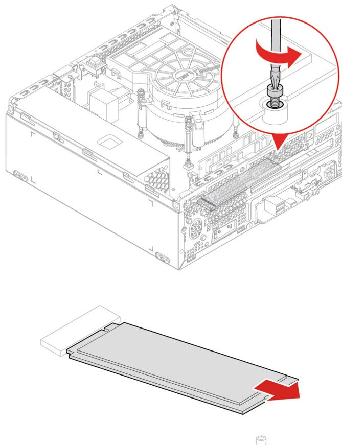
**Note:** If the card is held in place by retaining latch, press the latch as shown to disengage the latch. Then, gently remove the card from the slot.
