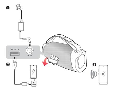
1 Charge the speaker before using it by opening the rear cover and connecting the speaker to the charging adapter.
