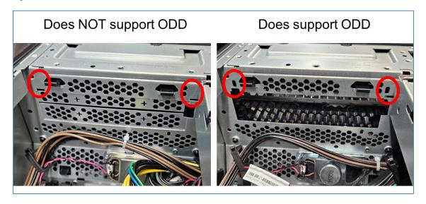
Systems with the ODD bracket installed will have some limitations to the maximum number of SATA drives. The bracket occupies the same space as the 3<sup>rd</sup> HDD and FASE, which would limit the maximum number of SATA drives to three.
