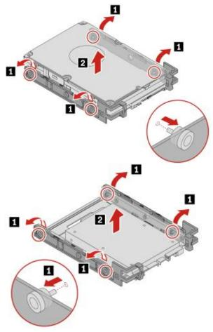
4. For 2.5" drives in the 3.5" adapter bracket, remove the screws holding the drive to the bracket.
