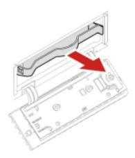
3. Remove the tray pins holding the SATA drive in each corner to separate the drive.
