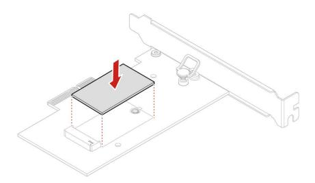
2. Insert the new M.2 solid-state drive into the M.2 slot. Then, insert the plug of the retention latch into the hole to secure the new drive.
