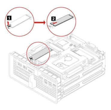
2. Reverse the steps to install a drive. For best drive performance when only one M.2 drive is installed in the system, install in Slot 1 as seen in the image below:
