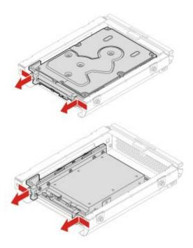
3. Remove the tray pins holding the SATA drive in each corner to separate the drive.
