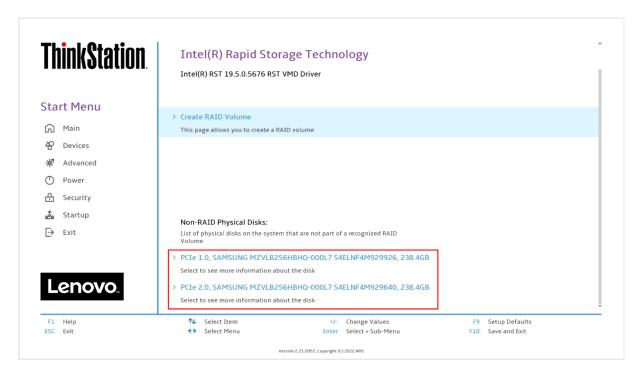
9. If all the disks installed are not shown as available, it may be necessary to clear any previous data from the disks. If no arrays have been created previously but there is an existing volume shown, it will be necessary to delete any previous arrays. Advance to step 15 to complete the process to delete any arrays. Return and proceed to step 10 once the desired drives are available.
