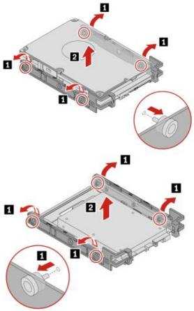
3. For 2.5" drives in the 3.5" adapter bracket, remove the screws holding the drive to the bracket.
