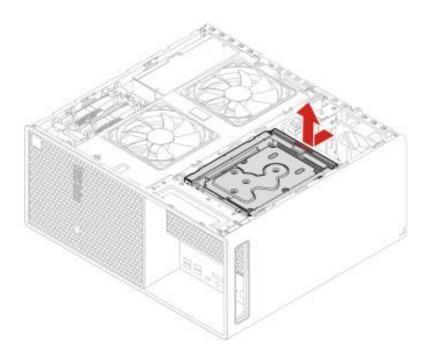
2. Pinch the handles of the drive tray and pull out of the drive cage.
