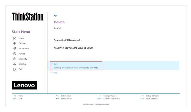
18. To verify the array was deleted, return the opening page of the "Intel(R) Rapid Storage Technology" and verify the drives are once again seen as available for the creation of a new array.
