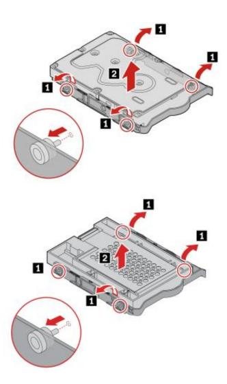
4. For 2.5" drives in the 3.5" adapter bracket, lift the metal tongue and push toward the back of the bracket. Lift the drive out of the adapter bracket and remove the metal frame from the drive.
