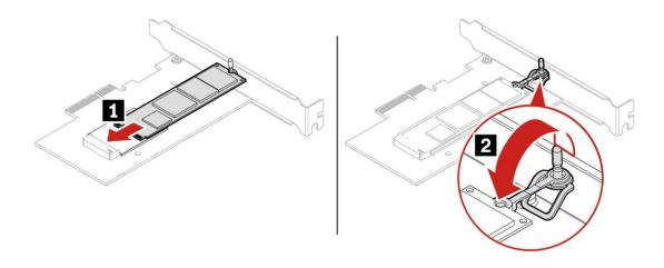
3. Position the heat sink on the M.2 solid-state drive PCIe adapter. Ensure that the two mounting studs in the heat sink are aligned with the holes in the M.2 solid-state drive PCIe adapter. Then, push the mounting studs downward to secure the heat sink to the adapter.
