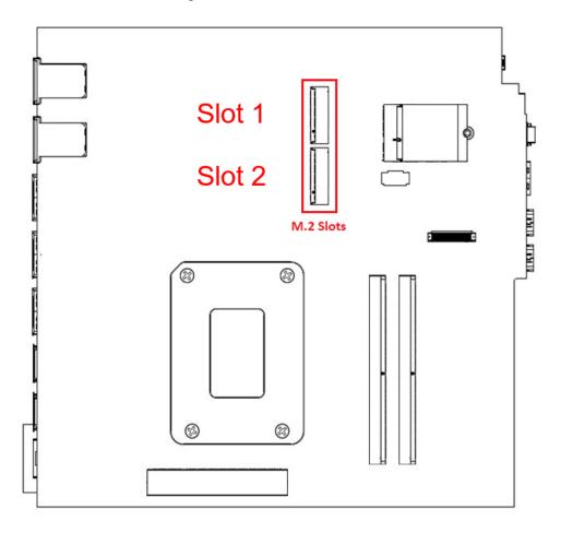
Figure 4 - P3 Ultra chassis with NVMe Callouts
