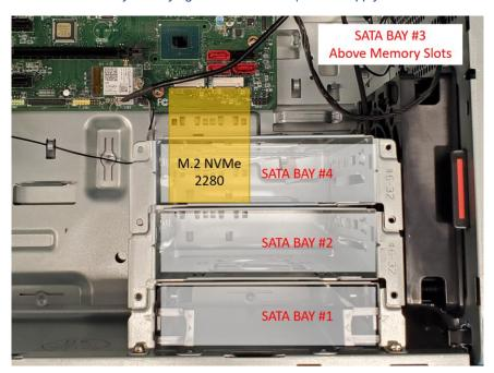
Additionally, in systems with a side fan assembly, the maximum number of SATA drives is three (See Figure 11) due to physical interference between the side fan assembly and SATA Bay 4. At the time of this writing, the side fan assembly is factory-fit on ThinkStation P3 Tower on all models with a 750W or 1100W PSU configured. It is not included in 500W PSU models.
