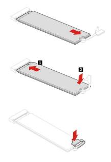
3. For best drive performance when only one M.2 drive is installed in the system, install in Slot 1 as seen in the image below:
