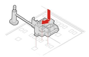
4. Install the heat sink with the bracket into the system.
