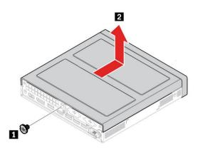
4. Turn the system over and slide the bottom plate towards the front of the system.
