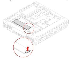
2. With the retention latch removed the M.2 SSD should lift slightly. If it remains attached to the heat sink pad underneath it, pull up on it gently until it is free of the pad. Slowly slide the M.2 horizontally away from the M.2 slot. To install the M.2 drive(s), reverse the procedure.
