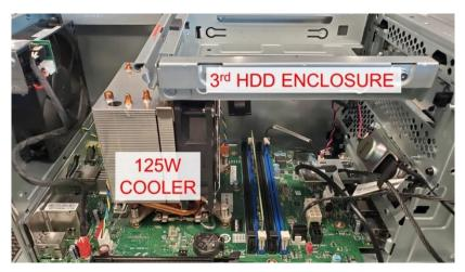
The use of four SATA drives will utilize all the available SATA ports on the motherboard. Adding additional SATA drives to the system may impact certain lengths of M.2 drives installed in the onboard M.2 slots. <u>SATA Bay</u> #4 & M.2 2280 drives will physically interfere and cannot be installed at the same time (See Figure 10).
