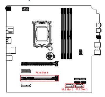
Figure 2 - P3 Tower Chassis with NVMe Callouts
