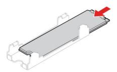
2. Remove the film that covers the thermal pad at the bottom of the heat sink, if any. Then, install the heat sink onto the M.2 drive in the bracket.
