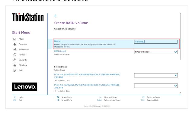
12. Select the drop-down box for "RAID Level" and select the desired RAID level. The RAID level options displayed are based on the type and number of drives available in the system.
