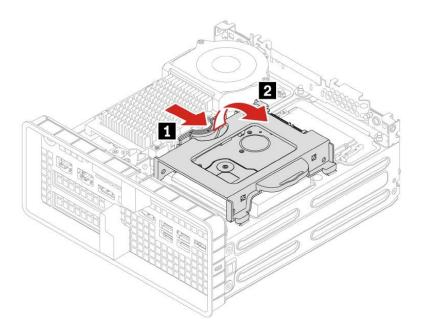
2. Gently stretch the drive carrier apart until the drive comes loose from the screw hole pins. Lift the drive up and out of the carrier.
