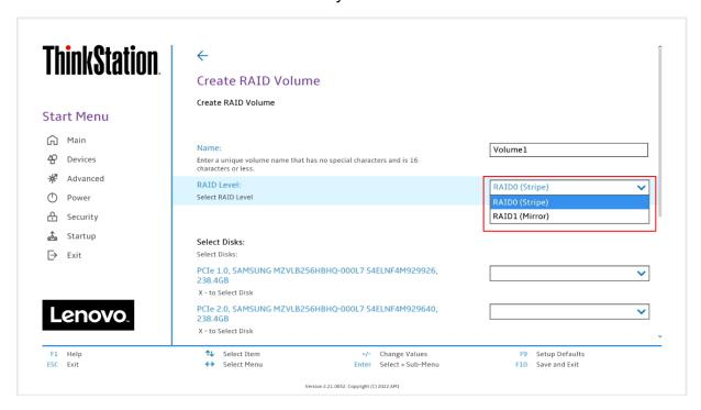
13. On the same page, select the drop-down box for each drive and select "X" to add the drive to the array. Once all the required drives are added, select "Create Volume". Unselected drives will appear in an OS like normal.
