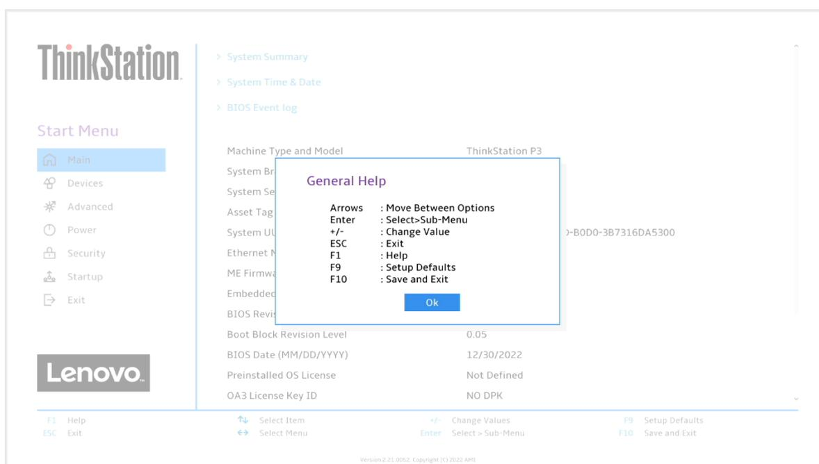
2. Select “System Summary” and scroll down to verify BIOS is recognizing all the drives installed in the system.
