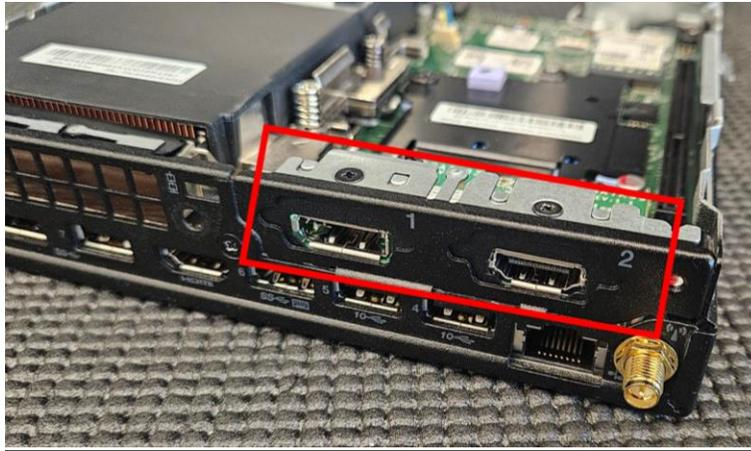
Figure 4, P3 Tiny Motherboard BTB Slots, Rear View
