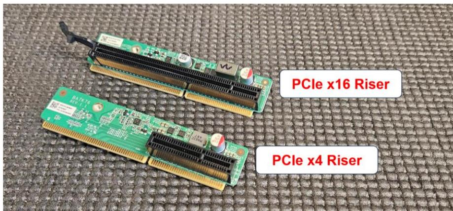
PCIe risers are installed at the factory based on system configuration. If no PCIe device is selected during initial purchase, no riser will be installed in the system. The part numbers for the risers are below. Additionally, an M3x6 screw is recommended to secure the riser to the side of the chassis.
