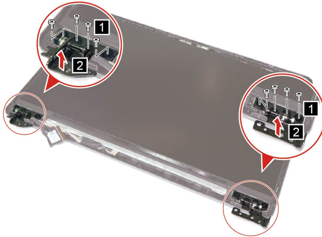
Figure 47. Remove eight screws and the hinges
