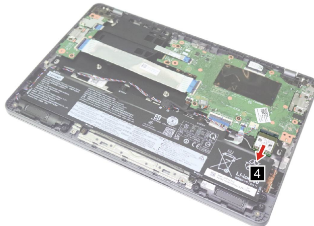
Figure 7. Remove the Wi-Fi card
