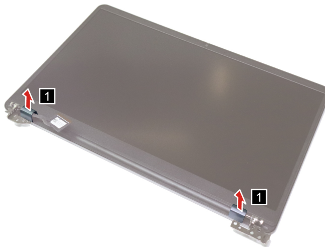
Figure 45. Remove the hinge caps
