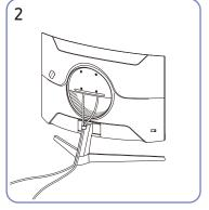
Put both cables in the cable holder on the stand (HOLDER-STAND CABLE) to organise the cables, as shown in the figure. Assembly is complete.
