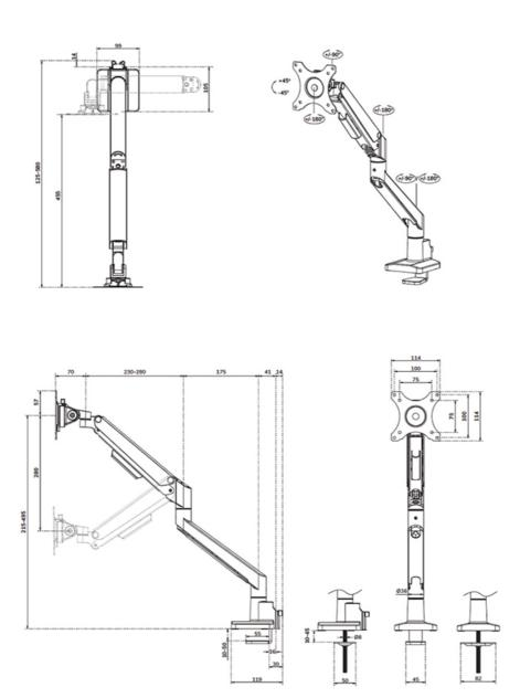
Neomounts Measuring unit: mm
