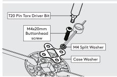
Attach the Bouncepad Case to its Mounting Arm. Take care to ensure correct & full thread engagement.
