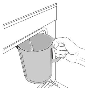
Once selected the "Drain" function, follow the actions indicated: Open the door and place a large jug under the drain nozzle located at the bottom right of the panel. Once started the draining, keep the jug in position until the operation is completed. The average duration for full load drainage is about three minutes.
