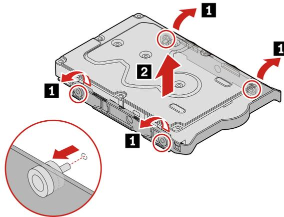
**Removal steps of the 2.5-inch primary hard disk drive, converter, and bracket**
