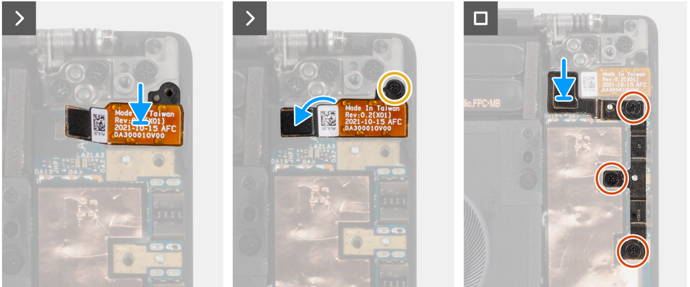
Figure 49. Installing the audio jack
