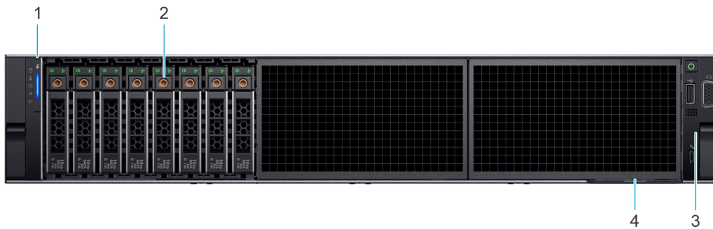
Figure 4. Front view of 8 x 2.5-inch NVMe drive system
