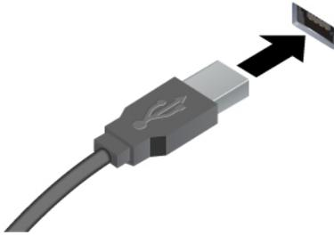
Connect USB-A compatible devices, such as a USB-A keyboard, USB-A mouse, USB-A storage device, or USB-A printer.
