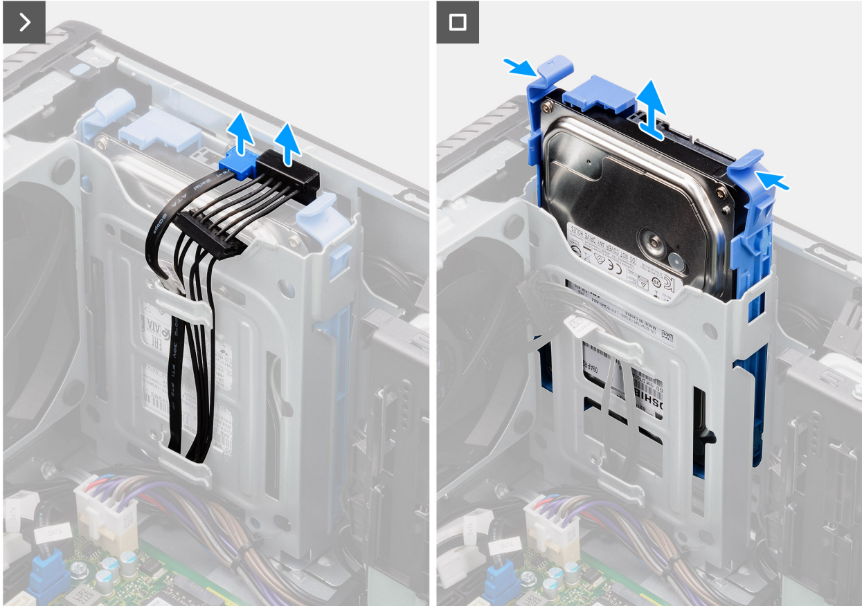
Figure 17. Removing the 3.5-inch hard drive assembly (Bay-2)
