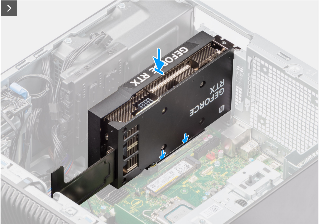
Figure 44. Installing the powered GPU
