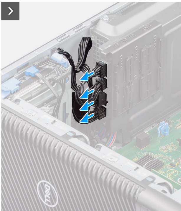
Figure 46. Removing the power-supply unit cover
