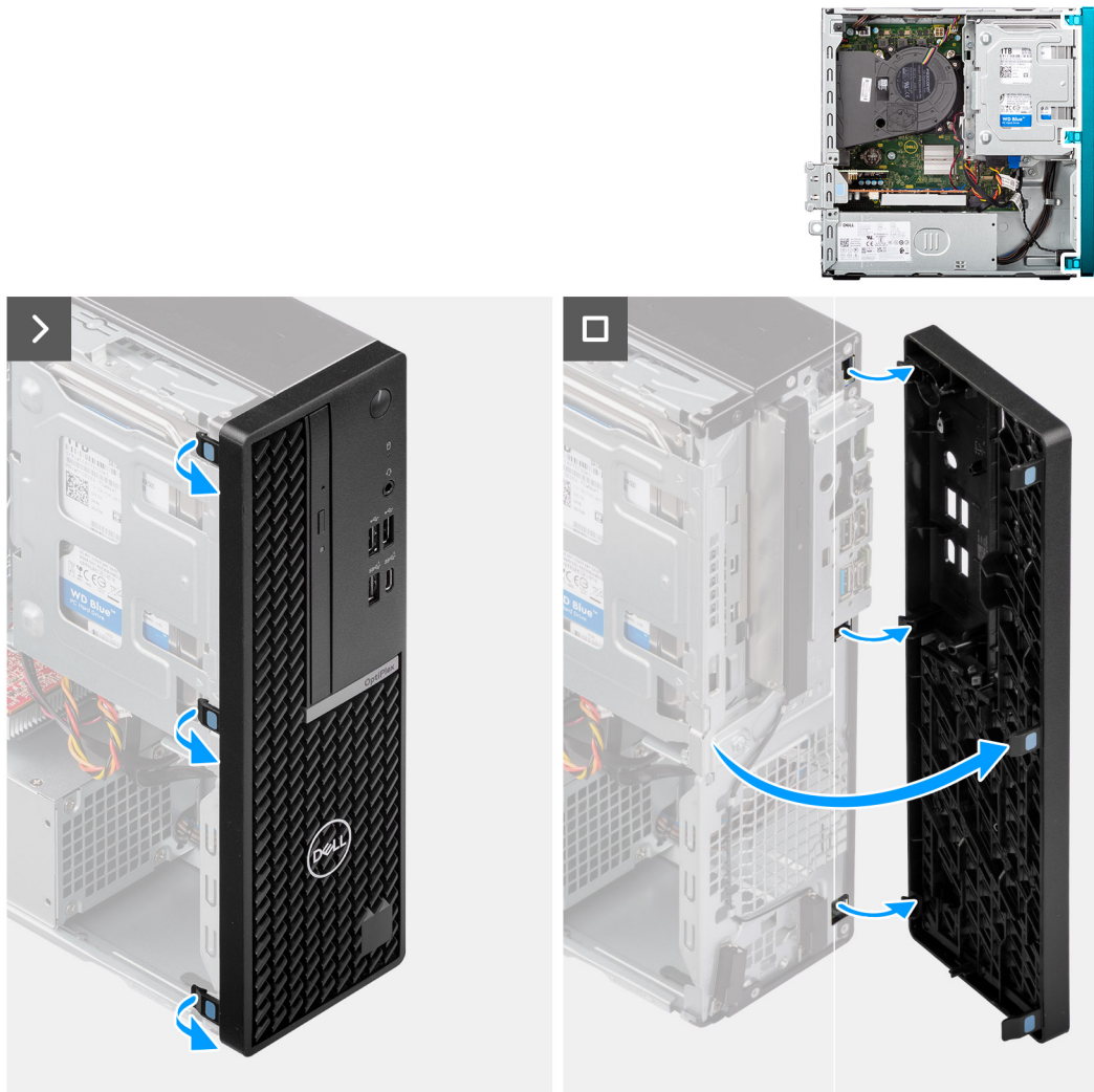
Figure 7. Removing the front bezel
