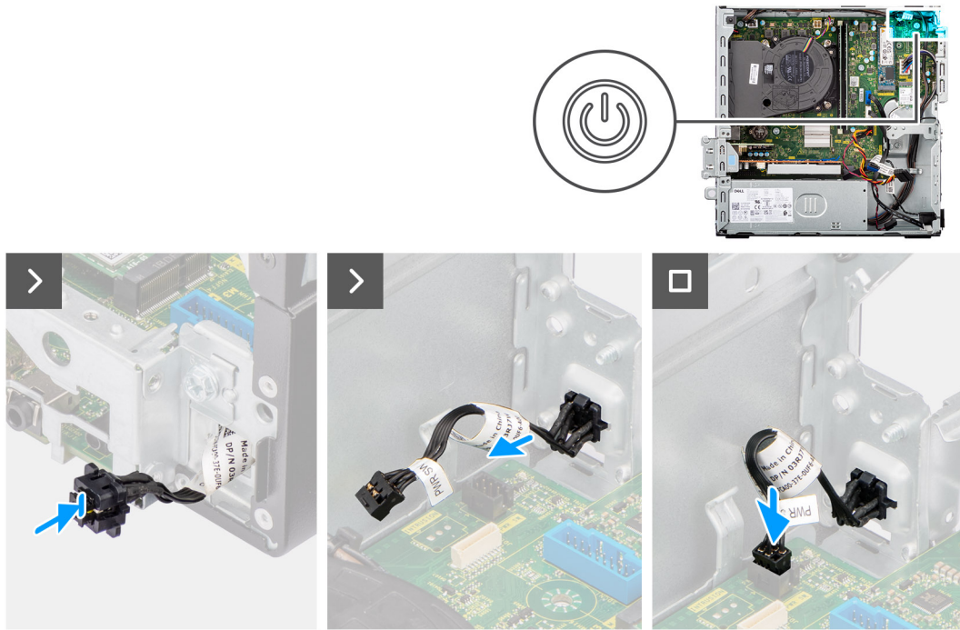
Figure 36. Installing the power button
