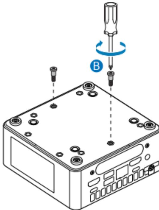
2. Attach the two slightly larger black screws to the bottom chassis cover of the Intel NUC.
