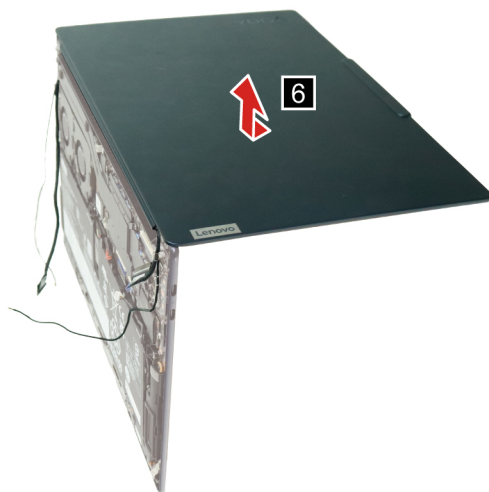
Figure 25. Remove the LCD module
