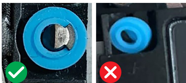
Figure 40. Seating position of the rubber grommets
