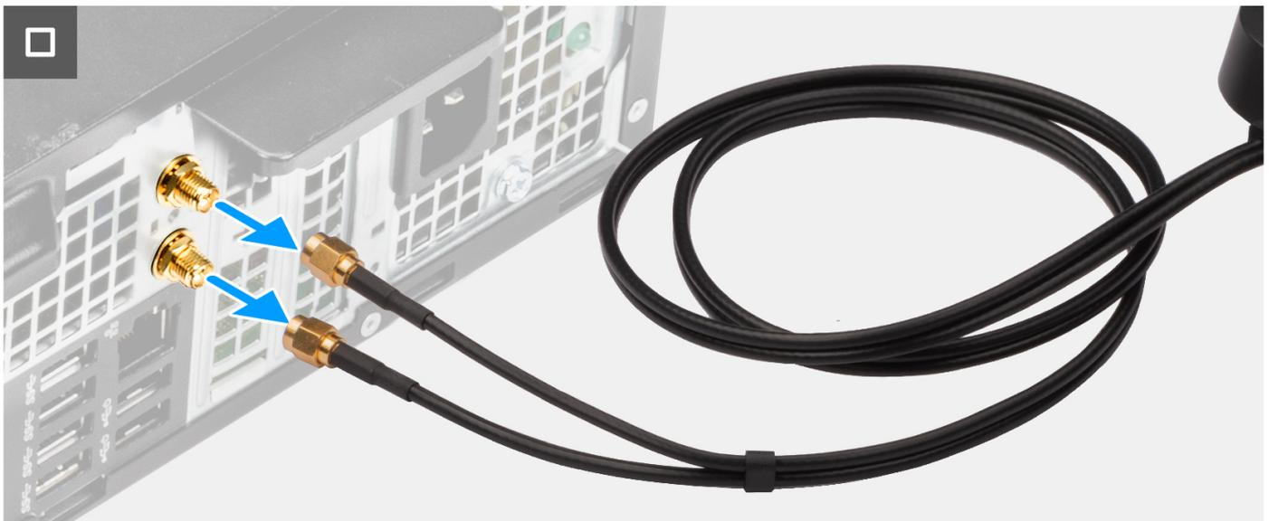
**Figura38. Remover a antena externa**
