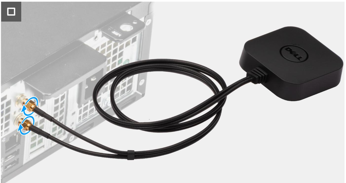
**Figura39. Instalar a antena externa**
