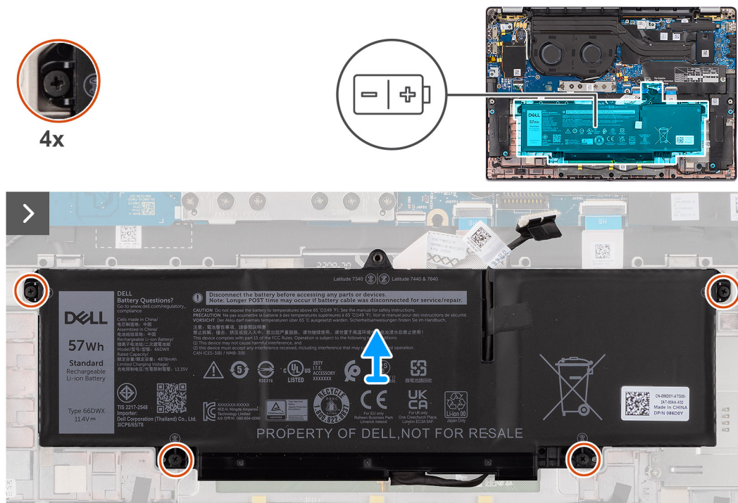
Figur 32. Ta bort 3-cellsbatteriet
