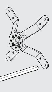
Position & mark were the **A1** VESA is to be located. Ensure the VESA is level.
