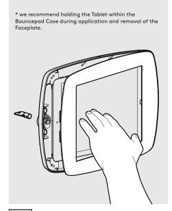
Locate & lock the Faceplate onto the 5 Bouncepad Case.
