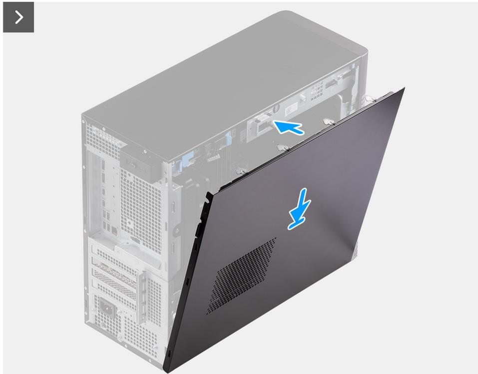
Figura10. Instalar a tampa lateral
