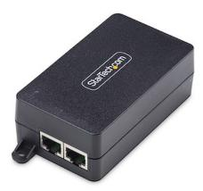
This 1-port multi-speed PoE+ Injector serves as a Power Sourcing Equipment (PSE) device and enables Ethernet speeds of 10Mbps, 100Mbps, and 1Gbps. This TAA-compliant mid-span inline injector can transmit network data and power up to 328ft (100m) for remote Powered Devices (PD).
