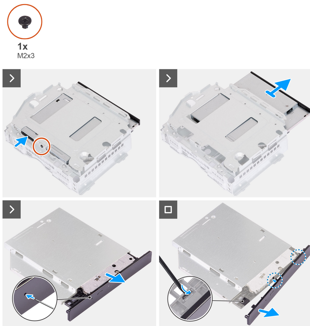
Figure 20. Removing the optical drive
