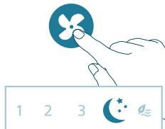
**Natural breeze mode (⾵):** Adjusts fan speeds up and down to mimic the natural movement of air and bring the refreshing feeling of an outdoor breeze into the room.
