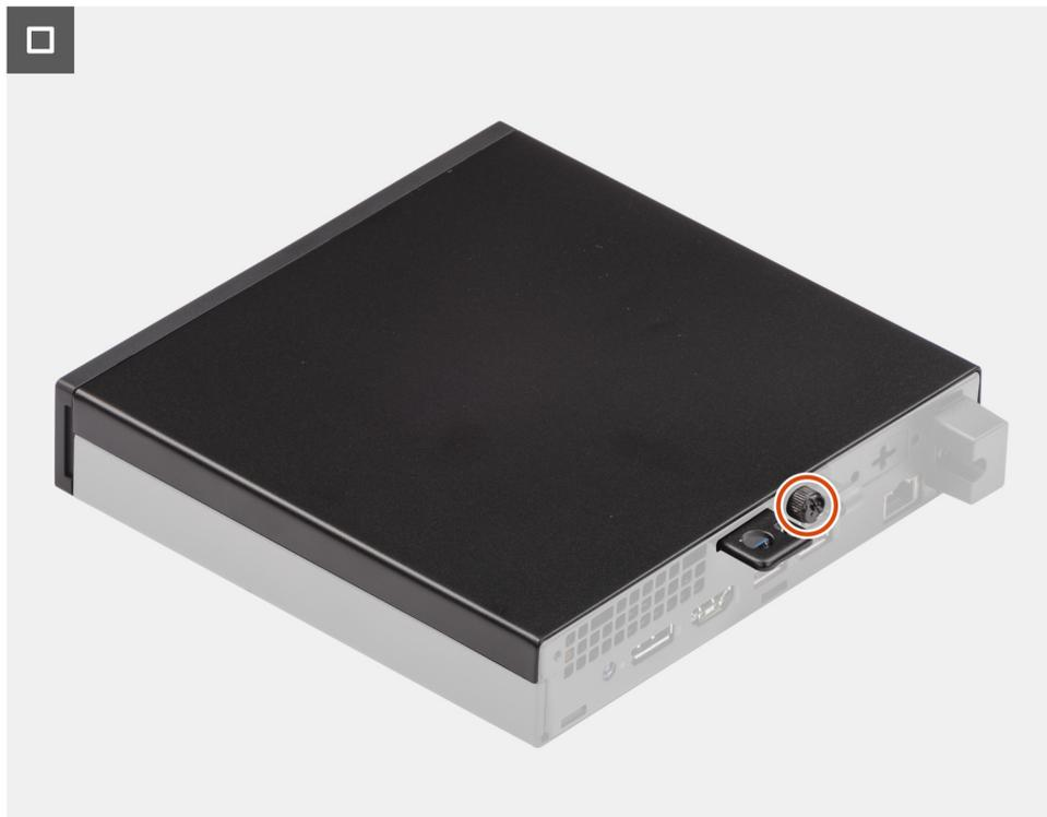
Figura12. Instalar a tampa lateral
