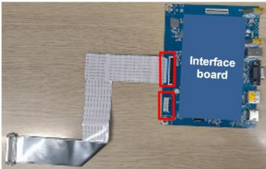
**S3** Assemble "Interface board" to "Main Shielding"
