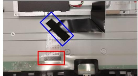
**S15** Unlock 13 screws to disassemble "Middle Frame" from "Panel"
