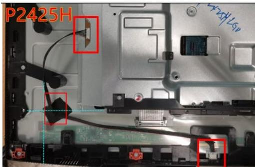
**S13** Tear off 3 conductive tapes from "Main Shielding" and "Panel"
