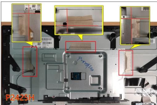
**S9** Insert "Backlight wire" to "Panel" and "Power Board"
