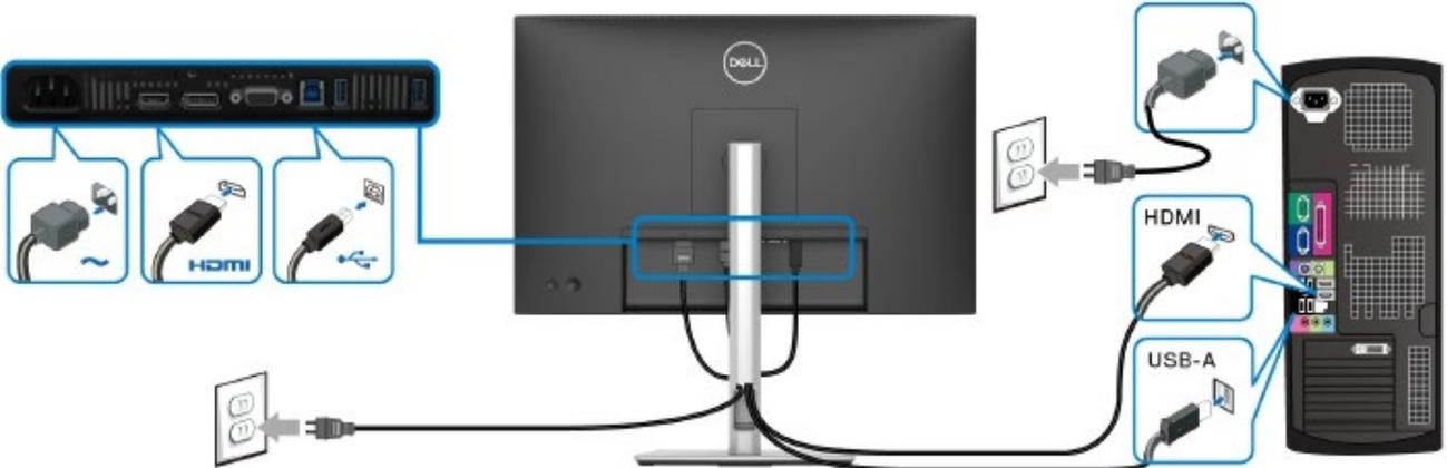
**Connect/ disconnecting the VGA cable (optional), USB 3.2 upstream cable and Power cable**
