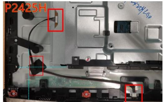
**S10** Assemble "USB board" with "USB Shielding"
