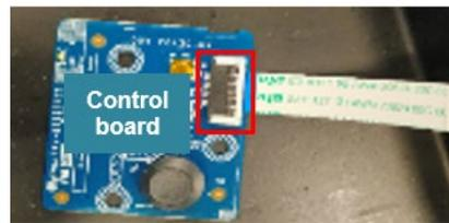
**S15** Assemble “Control board” to “Rear Cover”
