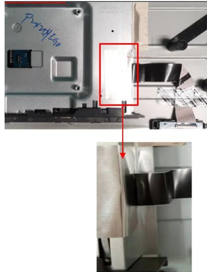
**S14** Insert “Control board FFC” to “Control board”
