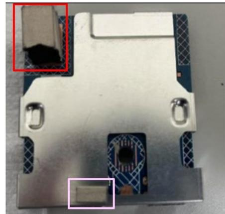
**S11** Disassemble "USB board" from "USB Shielding"
