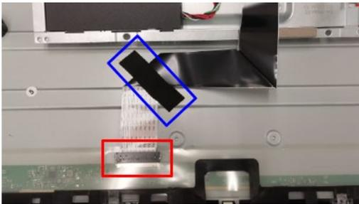
**S8** Attach 3 conductive tapes on "Main Shielding" and "Panel"
