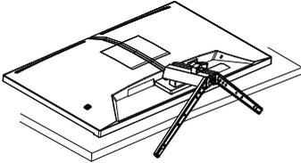
2. While keeping the release button pressed, tilt the base and slide it out.
