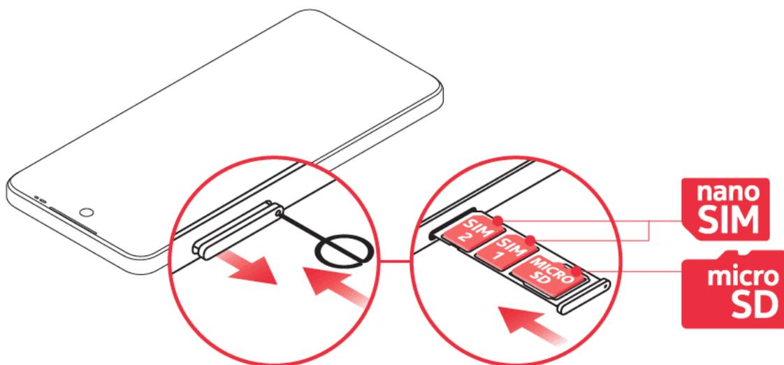
1. Open the SIM and memory card tray: push the tray opener pin into the tray hole and slide the tray out.
