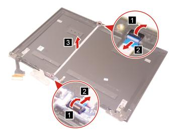
Figure 41. Disconnect and remove the camera cable
