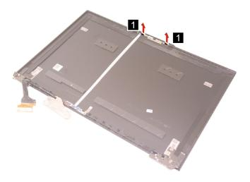
Figure 39. Remove the microphone rubbers
