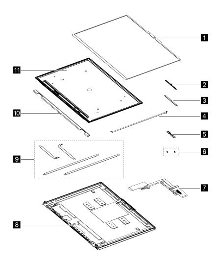
Figure 2. Exploded view - LCD
