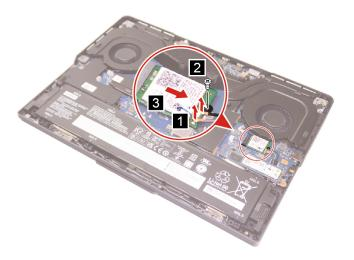
Figure 18. Remove the Wi-Fi card
