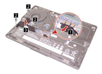
Figure 7. Remove the left SSD bracket
