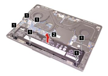
Figure 21. Remove the battery pack
