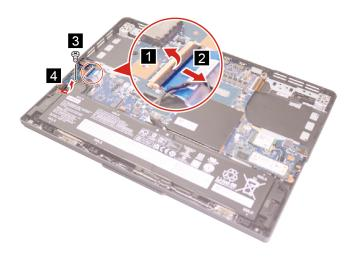
Figure 20. Remove the USB board
