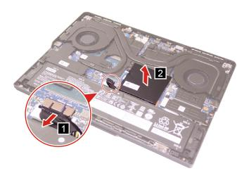
Figure 5. Remove the memory shielding
