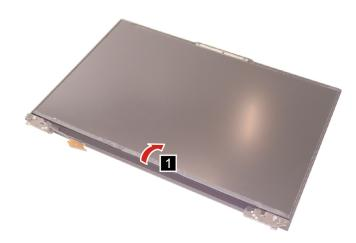
Figure 33. Remove the hinge cover
