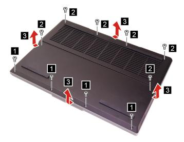
Figure 3. Remove the lower case
