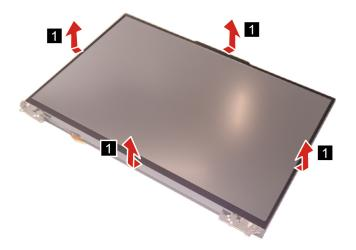
Figure 34. Remove the LCD bezel
