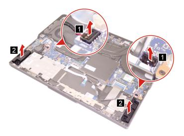
Figure 23. Remove the speakers
