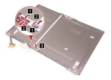
Figure 42. Disconnect cables and remove the sensor board
