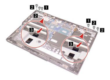
Figure 28. Remove six screws and open the latches
