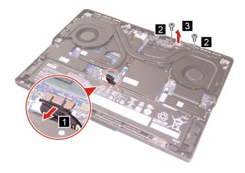
Figure 4. Remove the DC-in bracket
