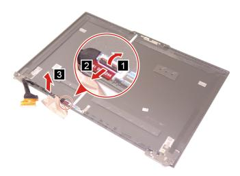
Figure 38. Remove the EDP cable
