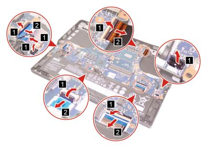
Figure 24. Disconnect cables
