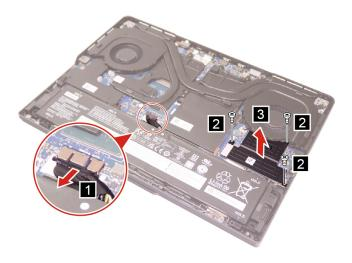
Figure 13. Remove the right SSD bracket
