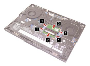
Figure 6. Remove the memory modules
