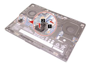
Figure 12. Remove the coin-cell battery
