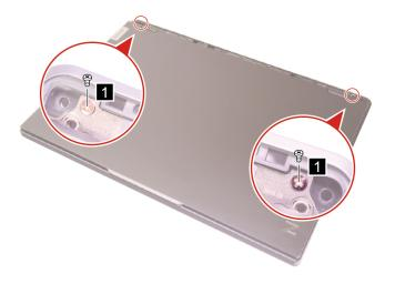
Figure 30. Remove two screws
