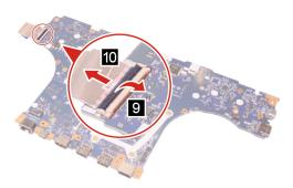
Figure 27. Remove the USB board cable
