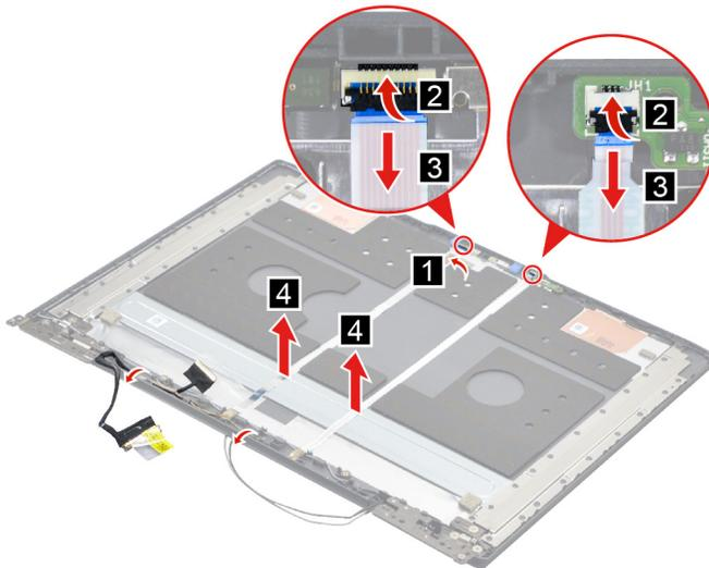
Figure 35. Remove the EDP cable
