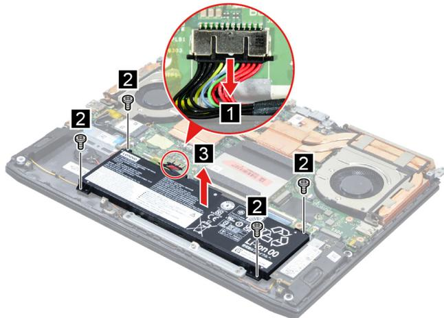
Figure 7. Remove the battery pack (on selected models)
