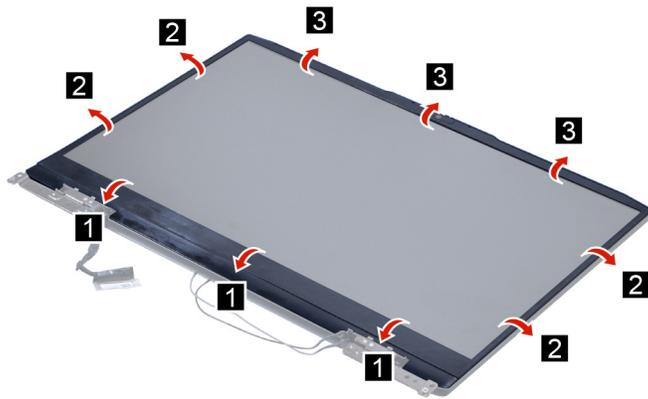
Figure 28. Remove the LCD bezel (on selected models)
