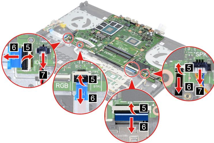
Figure 23. Disconnect cables connected to the system board
