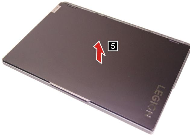
Figure 32. Remove the LCD unit
