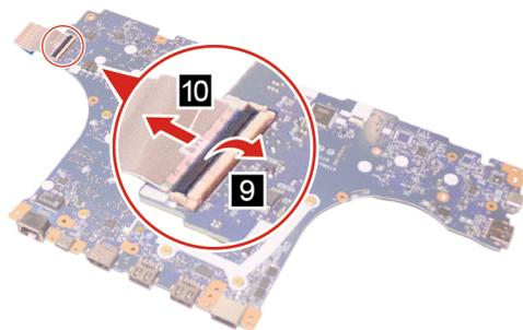
Figure 27. Remove the USB board cable
