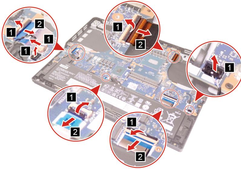
Figure 24. Disconnect cables
