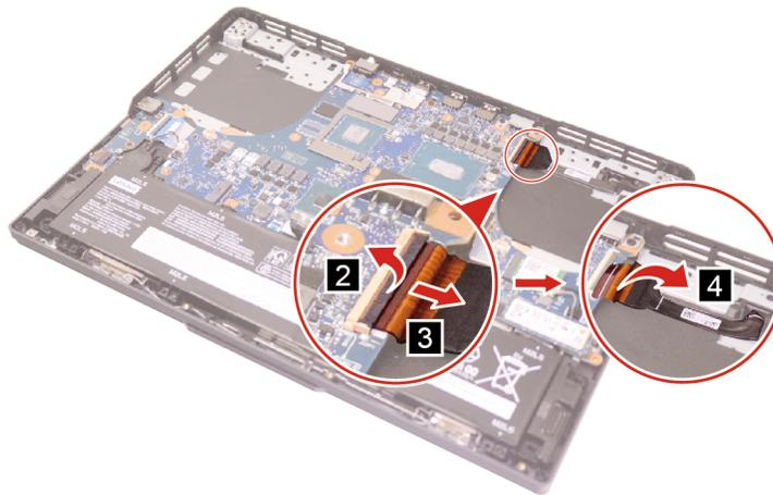
Figure 31. Disconnect and lift the EDP cable
