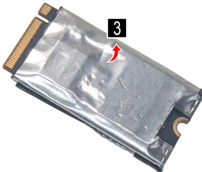
Figure 19. Remove the solid-state drive foil
