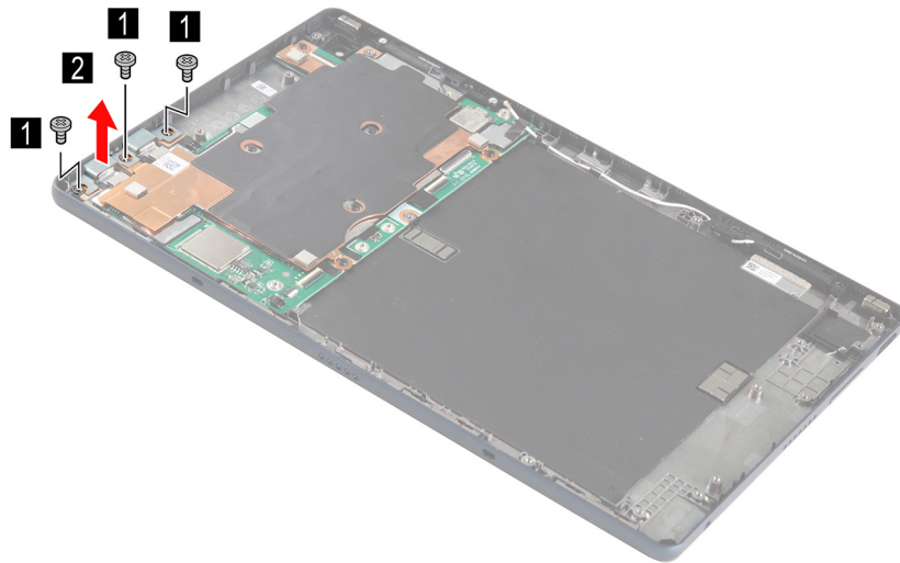
Figure 22. Remove three screws and the Type-C bracket
