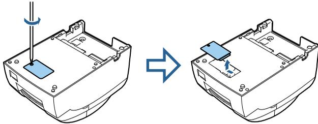
3. Use an object with a thin tip to set DIP switch settings.
