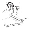
**4.** Remove filter: Lay a cotton cloth beneath the water filter, which can absorb a small amount of rest water. Then remove the water filter by turning it out anticlockwise.
