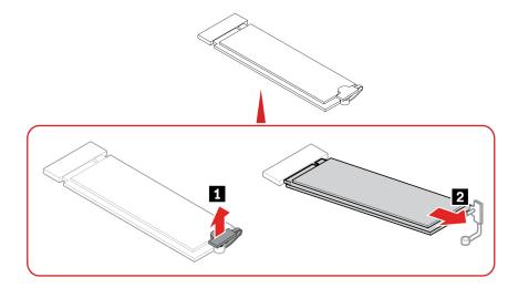
**Note:** Remove the film that covers the thermal pad (if any) when installing the M.2 solid-state drive.
