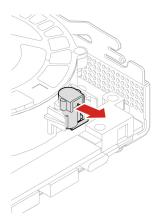
3. Disconnect the system fan cable from the system fan connector on the system board.
