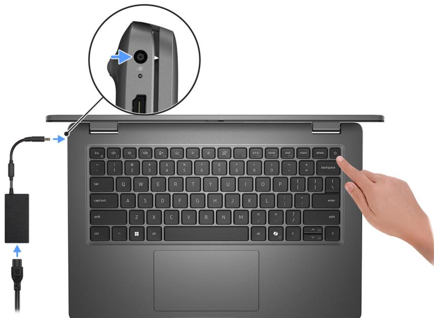
**Figure 1. Connect the power adapter and press the power button.**
