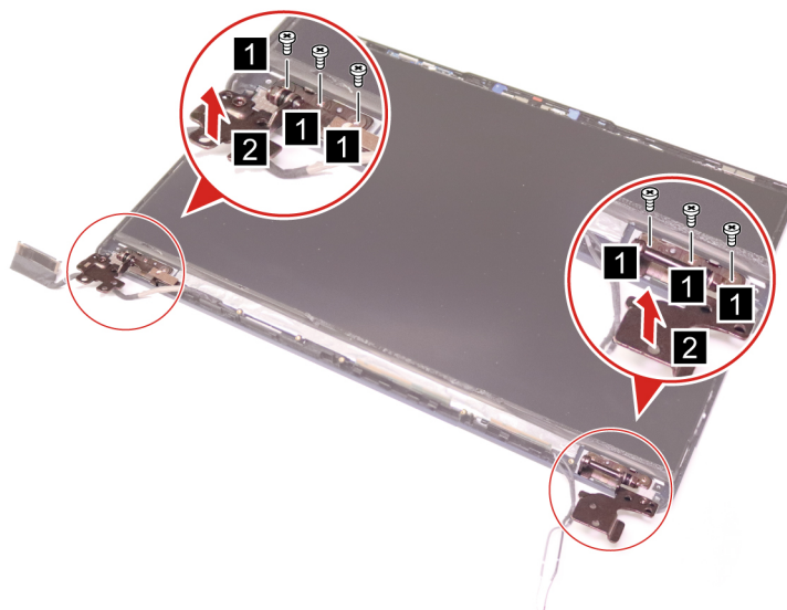
Figure 36. Remove six screws and the hinges
