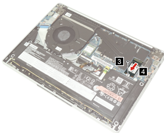
Figure 11. Remove one screw and the solid-state drive
