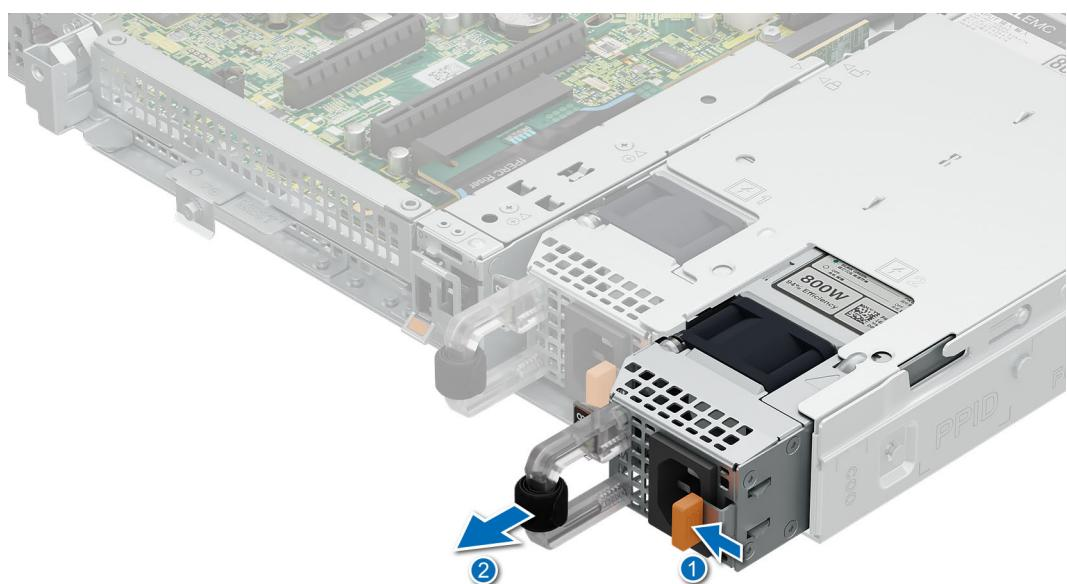
**Figure 73. Removing a power supply unit**
