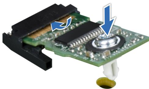
Figure 79. Installing the TPM
