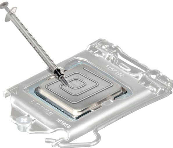
**Figure 48. Applying thermal grease**
