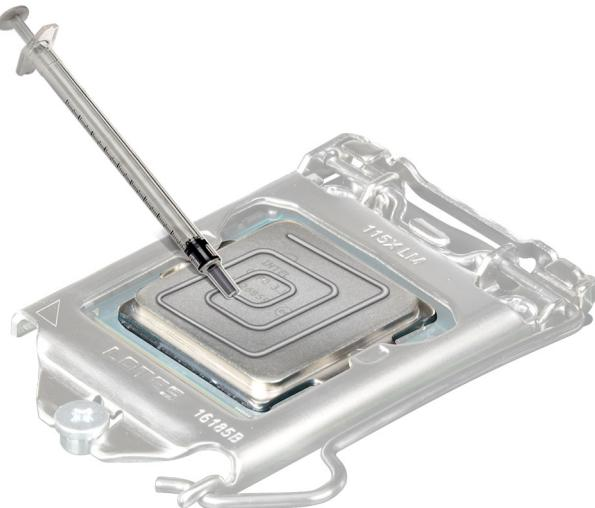
**Figure 47. Applying thermal grease**
