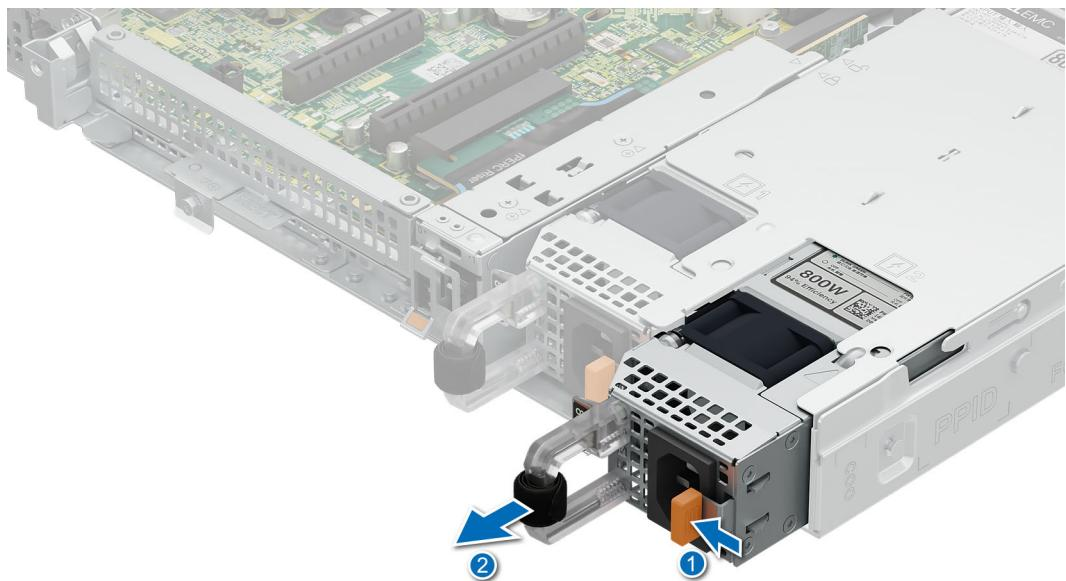
**Figure 74. Installing a power supply unit**
