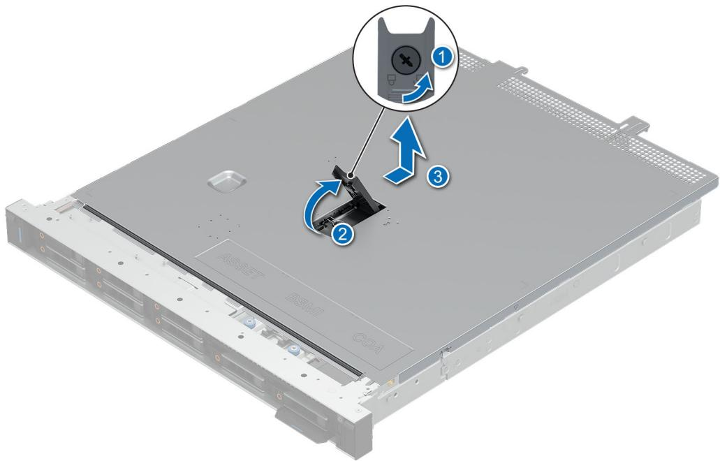
**Figure 16. Removing the system cover**
