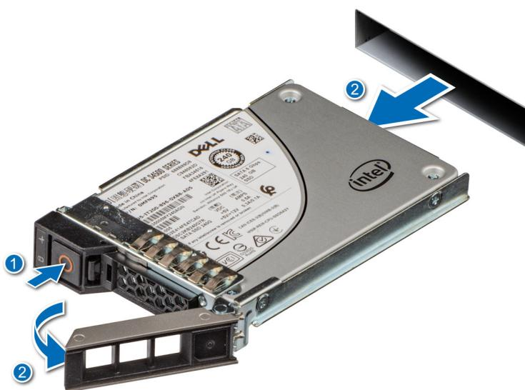
**Figure 35. Removing a drive carrier**
