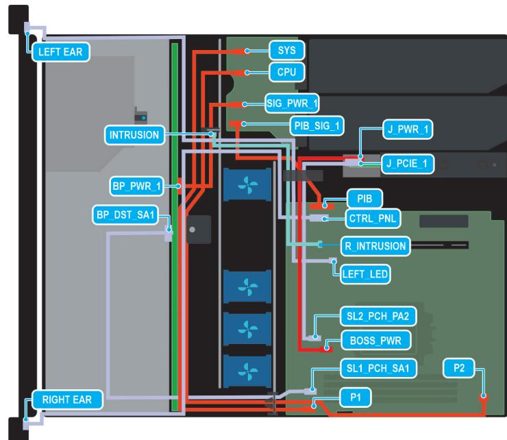
**Figure 28. Configuration 0: 4 x 3.5 inch SATA with BOSS N1 (optional)**
