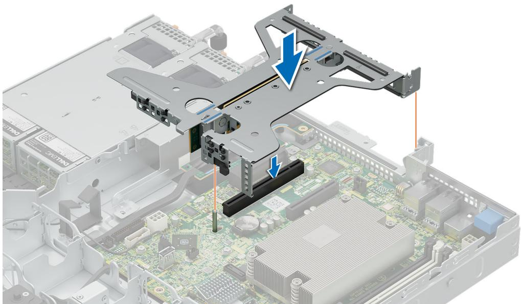
**Figure 54. Installing the riser**
