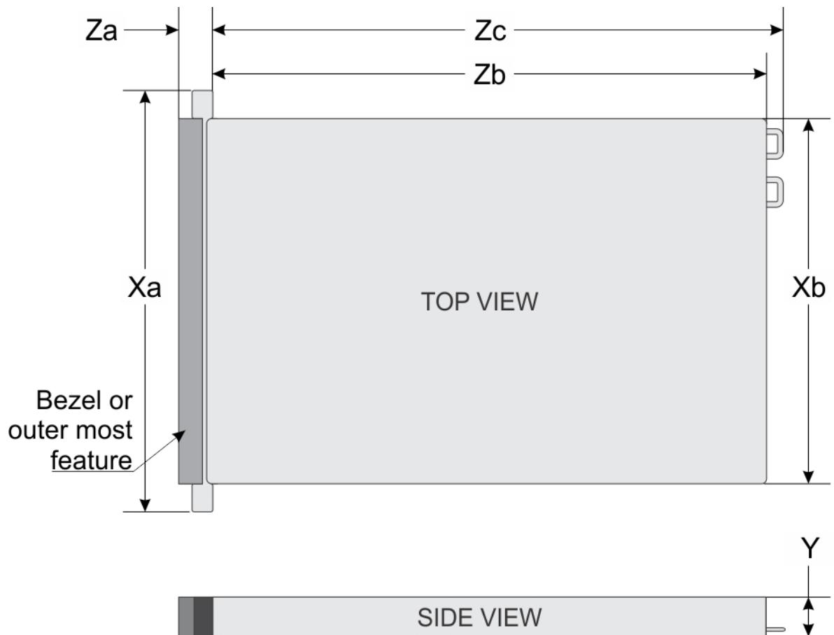
Figure 12. Chassis dimensions
