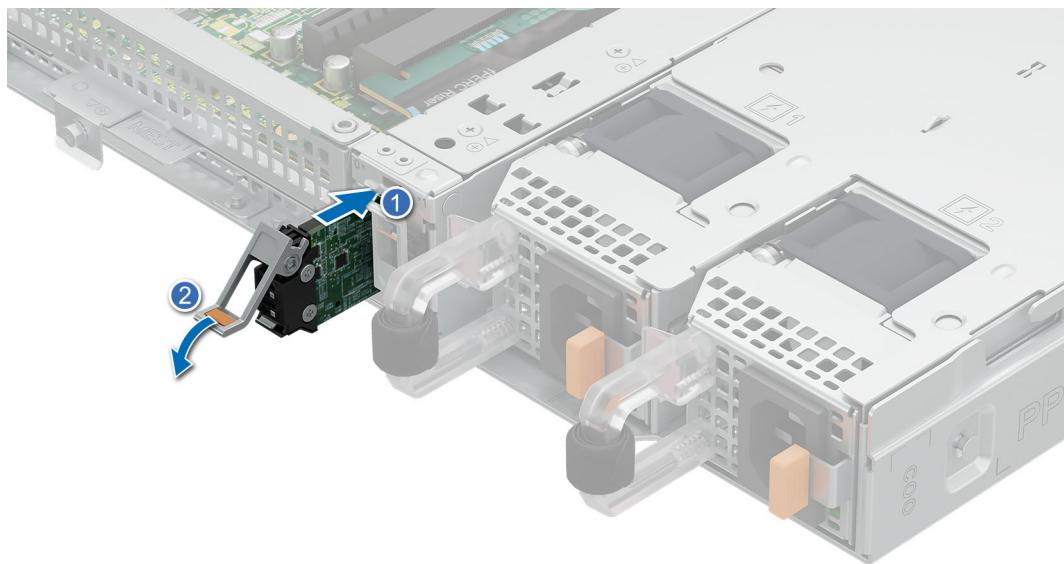
**Figure 60. Installing the BOSS N1 M.2 module**
