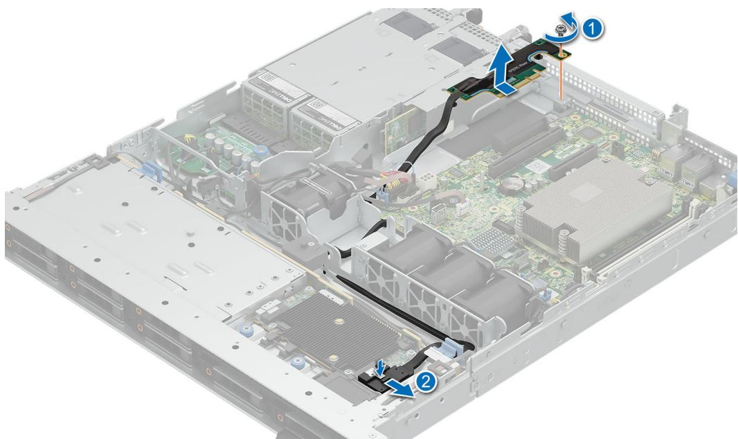
**Figure 68. Removing the front PERC card riser**
