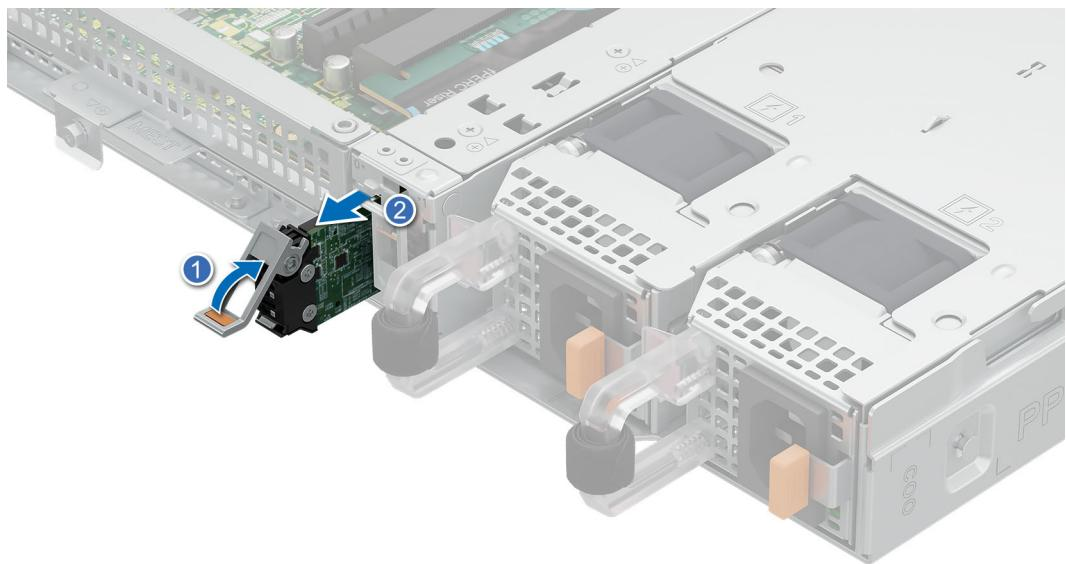
**Figure 55. Removing the BOSS N1 M.2 module**
