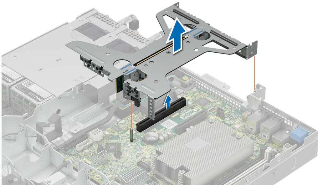
**Figure 53. Removing the riser**
