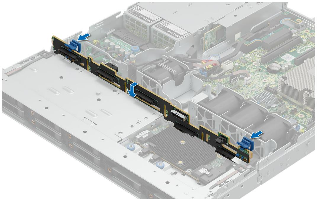
**Figure 27. Installing front drive bay backplane**
