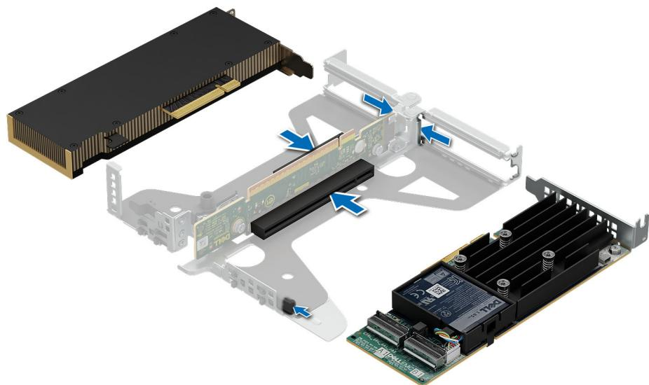
**Figure 52. Installing expansion card into the riser**
