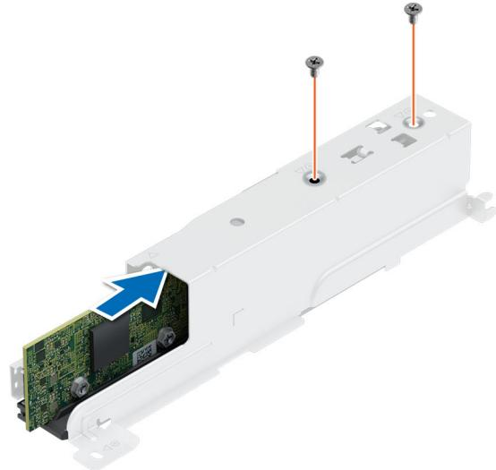
**Figure 58. Installing the BOSS N1 card**
