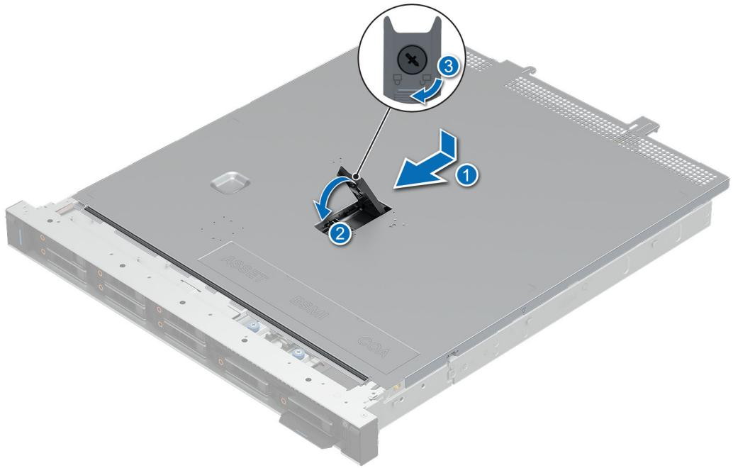
**Figure 17. Installing system cover**
