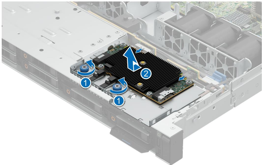
**Figure 67. Removing the front PERC card**
