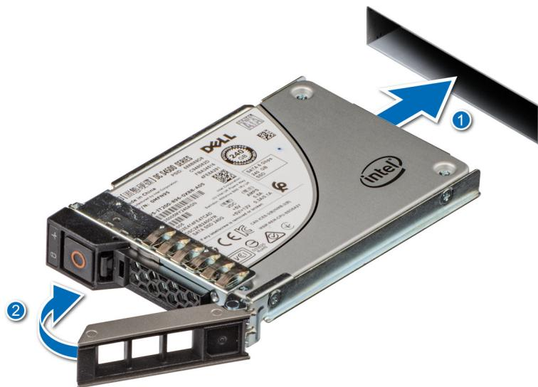
**Figure 38. Installing a drive carrier**
