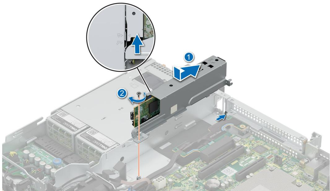
**Figure 59. Installing the BOSS N1 cage**
