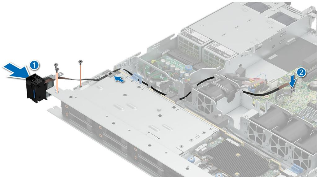
**Figure 82. Removing the left control panel**
