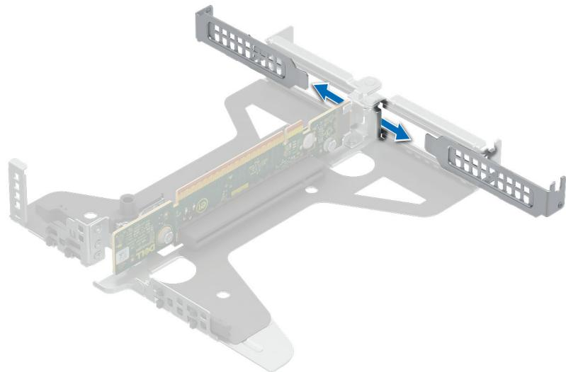
**Figure 51. Removing filler bracket from the riser**
