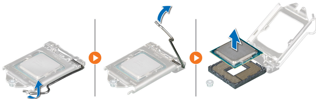
Figure 53. Removing the processor
