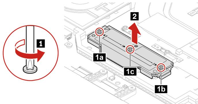
**Note:** When removing the top cover, ensure you lift it vertically as shown below.
