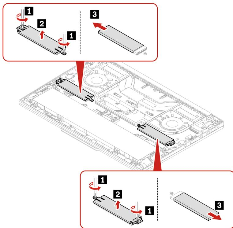
Step 2. Install the M.2 solid-state-drive and M.2 solid-state drive bracket in reverse order.
