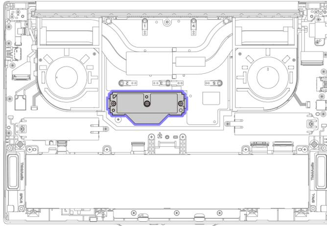
Step 1. Remove the memory module as shown below.
