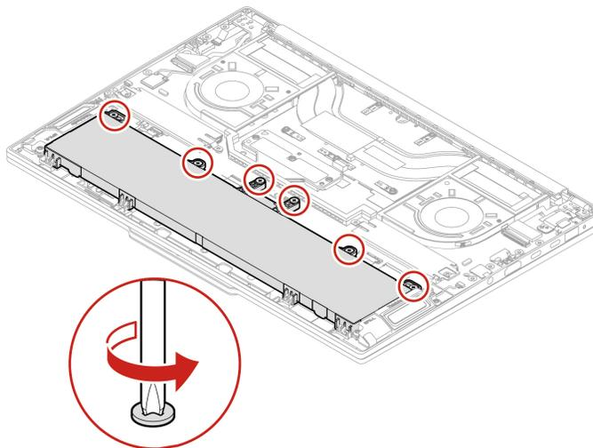
b. Remove the battery as shown below.
