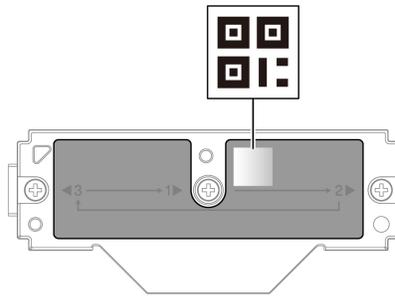
Step 1. Remove the top cover as shown below. Ensure you loosen screws in alphabetical order.
