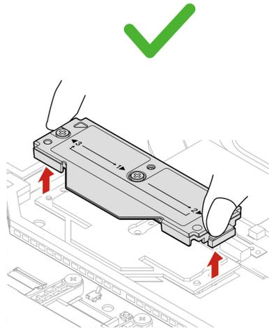
Step 2. Install the top cover as shown below.
