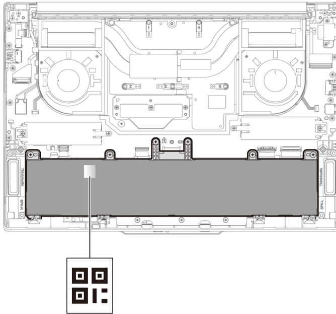
Step 1. Remove the built-in battery as shown below.
