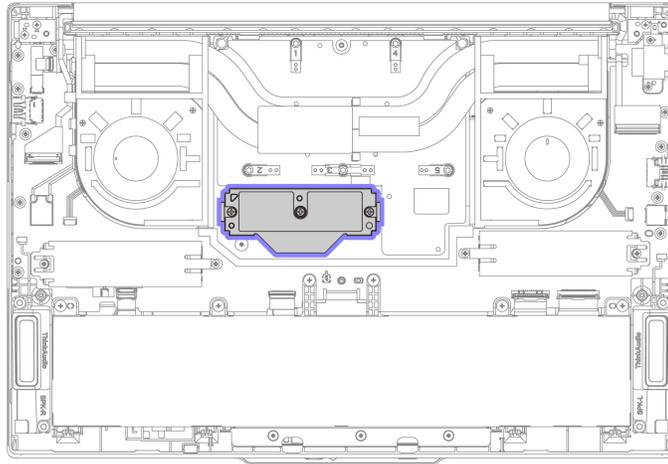
Step 1. Remove the connector as shown below.
