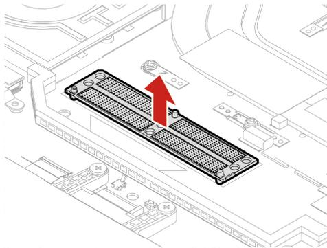
Step 2. Install the connector as shown below.
