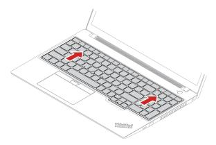
3. Pivot the keyboard slightly upward **1** and then turn over the keyboard **2**.
