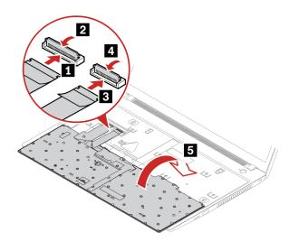
2. Insert the keyboard into the keyboard bezel as shown. Ensure that the top edge of the keyboard (the edge that is close to the display) is under the keyboard bezel.
