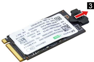
Figure 15. Remove the SSD bracket
