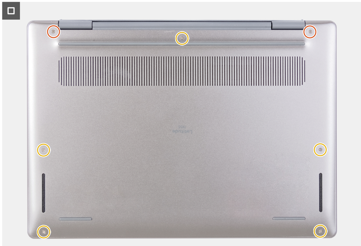
Figure 20. Tightening and replacing the screws
