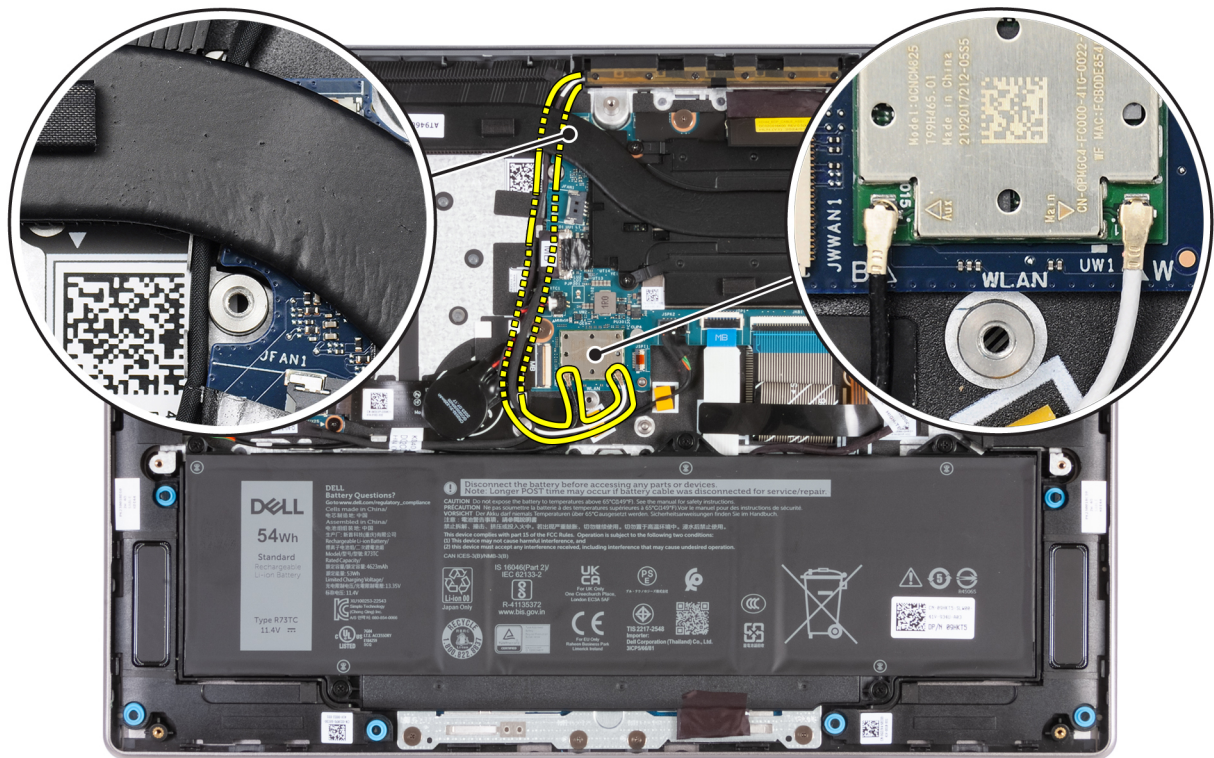
Figure 62. Installing WLAN-antenna cables
