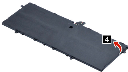
Figure 6. Peel off the battery mylar
