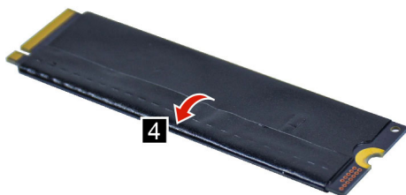
Figure 9. Remove the SSD mylar
