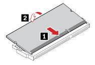
Note: During the installation, ensure that you align the memory module to the slot and press down on both ends until the latches are fully engaged with a click.
