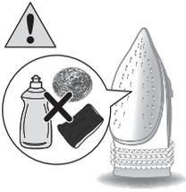
Note: To keep the soleplate smooth, avoid hard contact with metal objects. Never use a scouring pad, vinegar or other chemicals to clean the soleplate.
