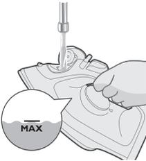
5 Fill water tank up to the MAX indication in the water tank.
