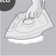
ECO setting: Minimum constant steam is delivered continuously for garments with less creases. This setting also saves energy.
