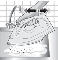
**11** Continue to shake the iron until all the water in the water tank has been released.
