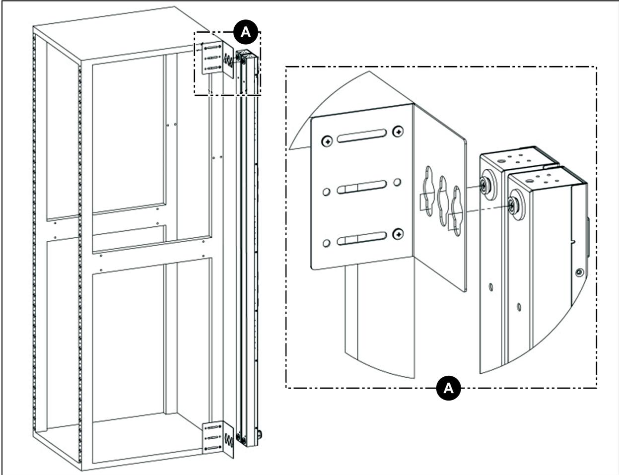
Figure 3.7 Offset/Side Mount Brackets
