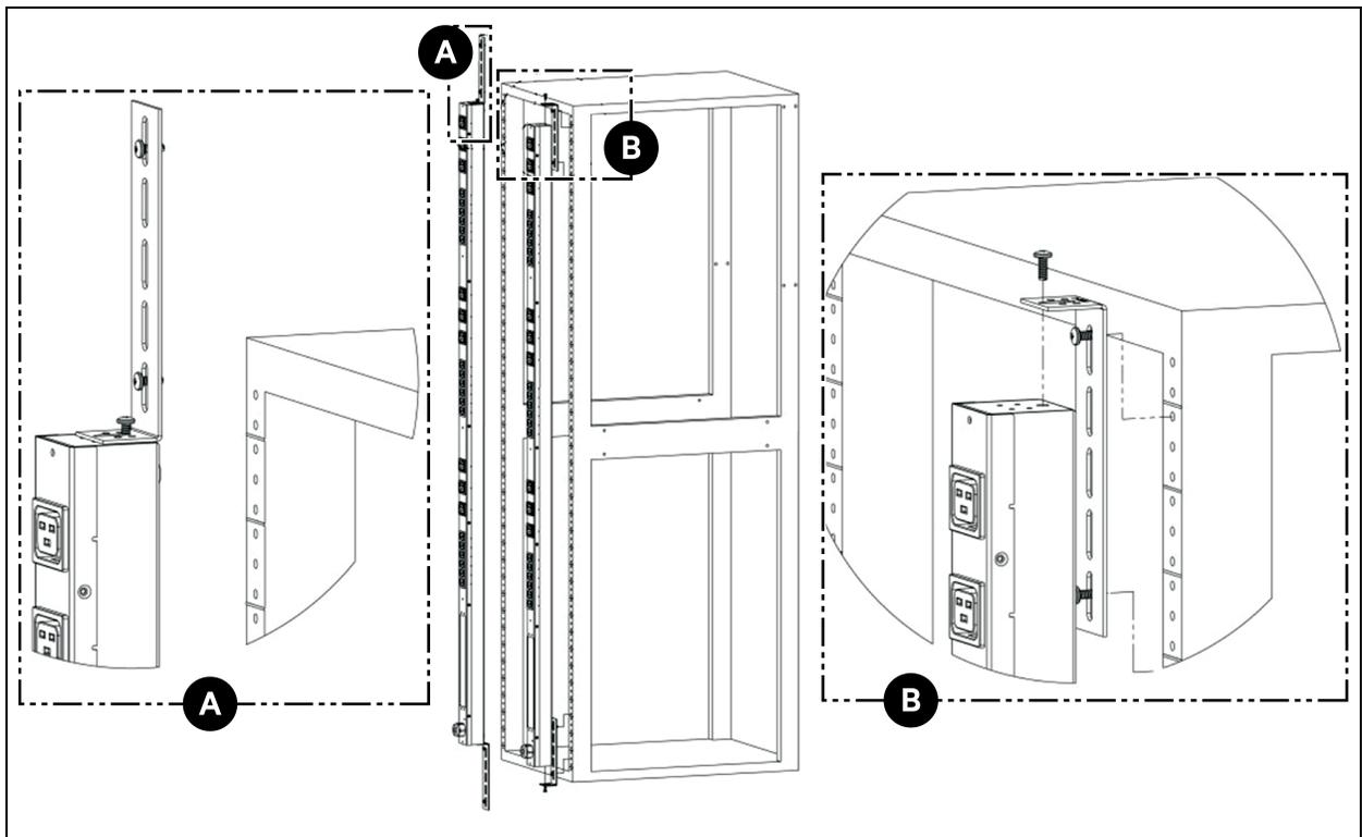
Figure 3.4 Toolless Mounting Hardware
