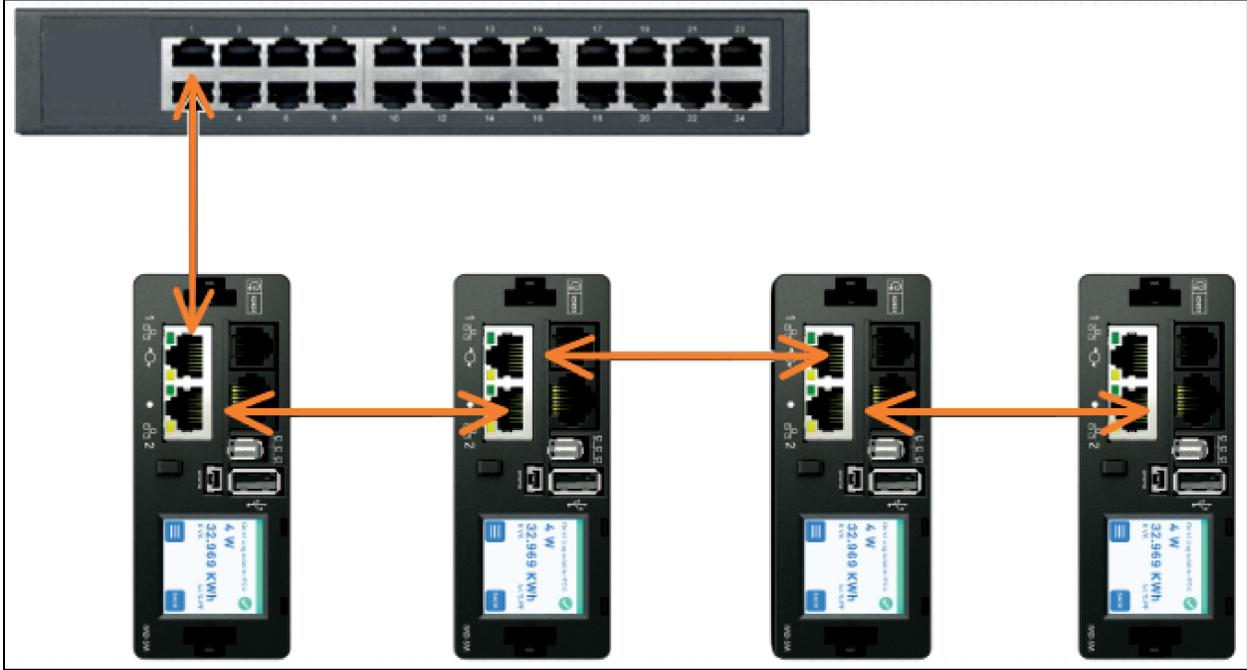
**Fault Tolerant Daisy-Chaining**
