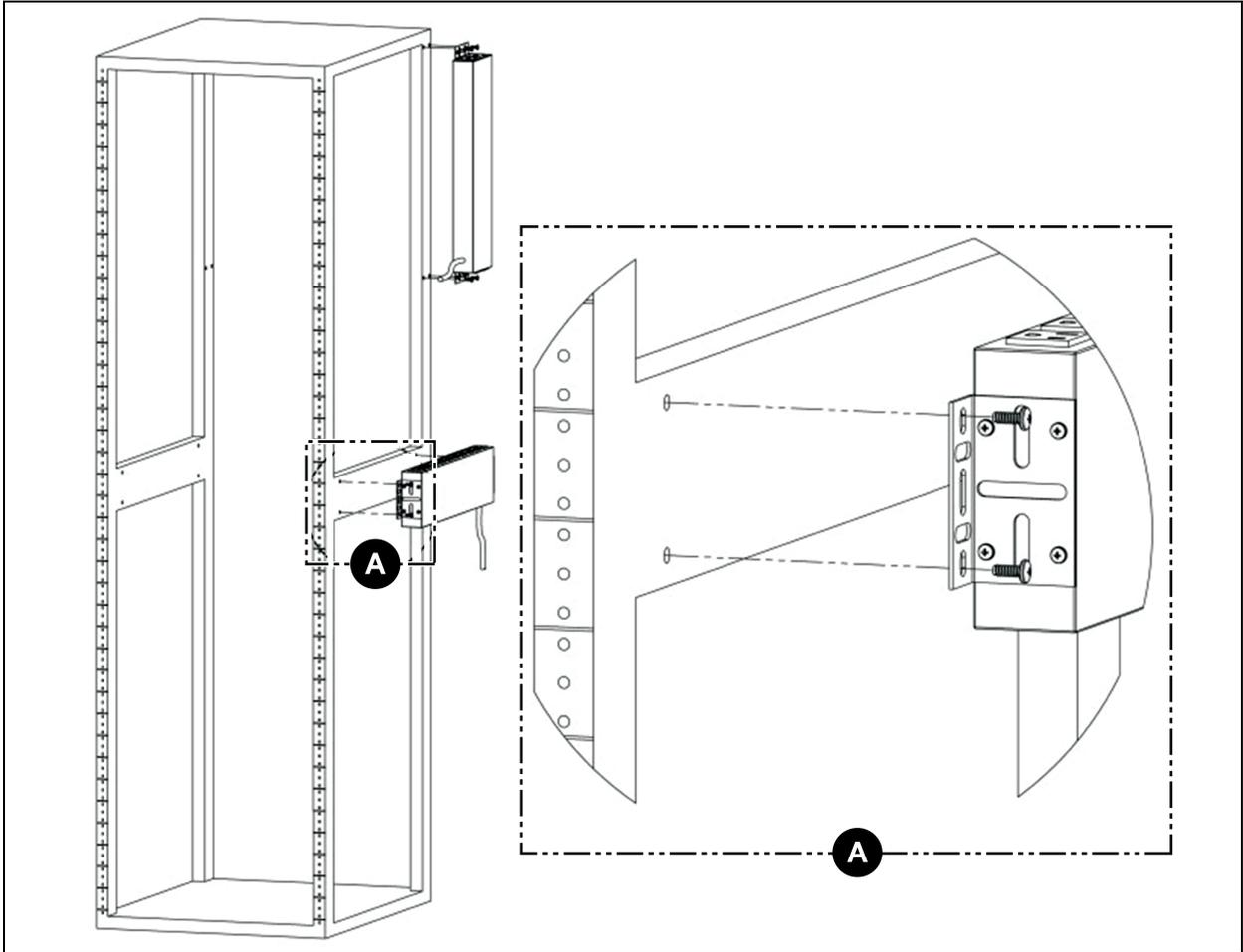
Figure 3.12 23" (inch) Conversion Mount Brackets
