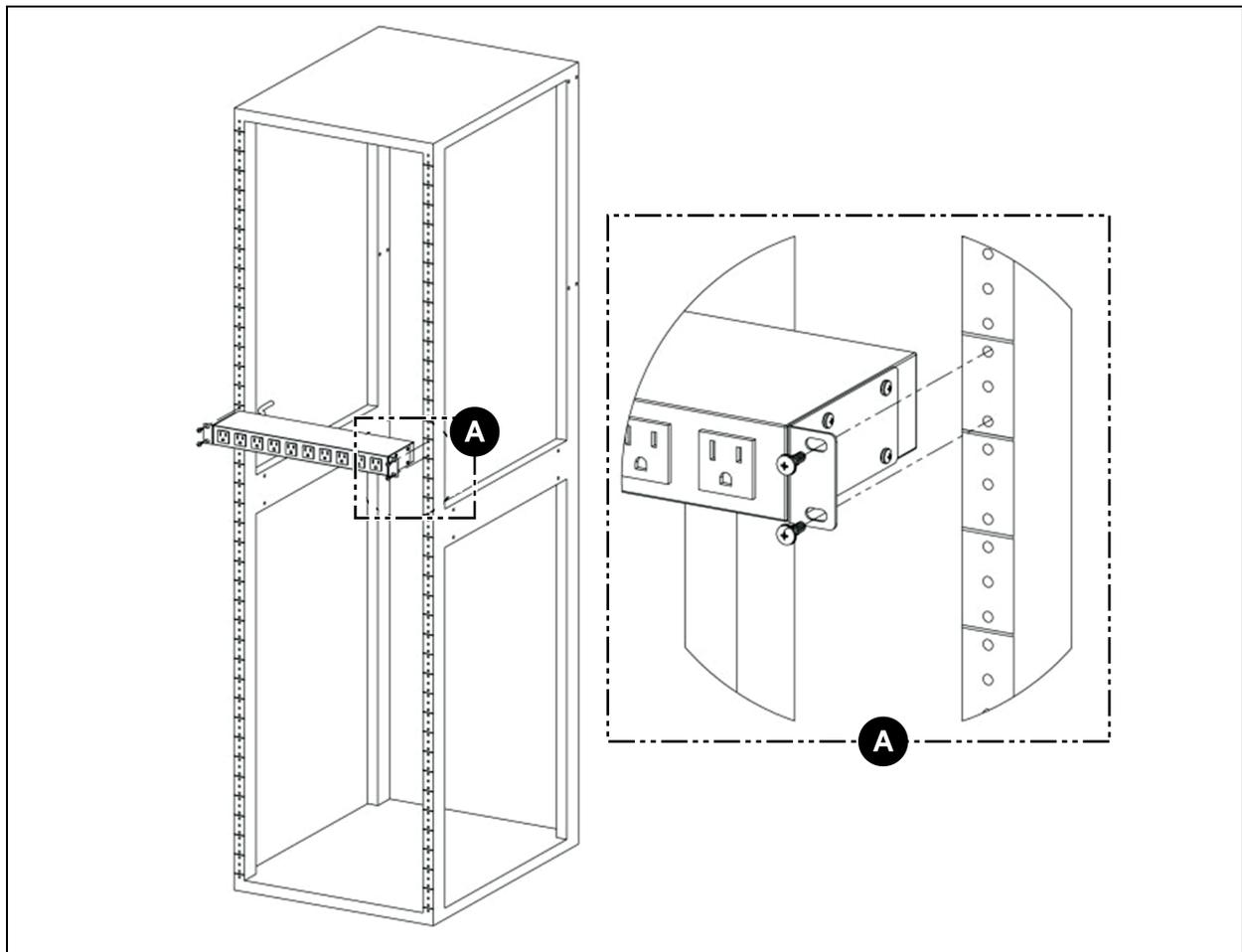
Figure 3.10 Adjustable Mount Bracket
