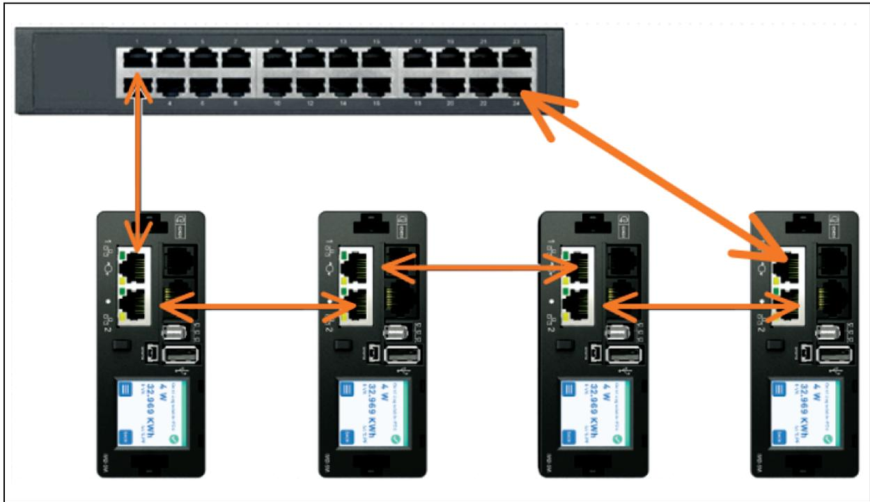
When both network interfaces are connected, the IMD implements a network bridging protocol called the Rapid Spanning Tree Protocol (RSTP). RSTP is an IEEE standard that is implemented by all managed bridges. Using RSTP, bridges in the network exchange information to find redundant paths or loops. IPv6 should be disabled when using redundant network connectivity.
