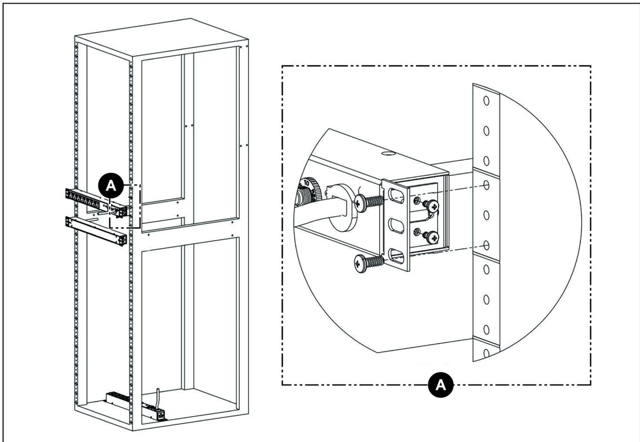
Figure 3.14 Mount Brackets for Vertiv™ Geist™ Universal Power Distribution Unit (UPDU) with Pivoting End
