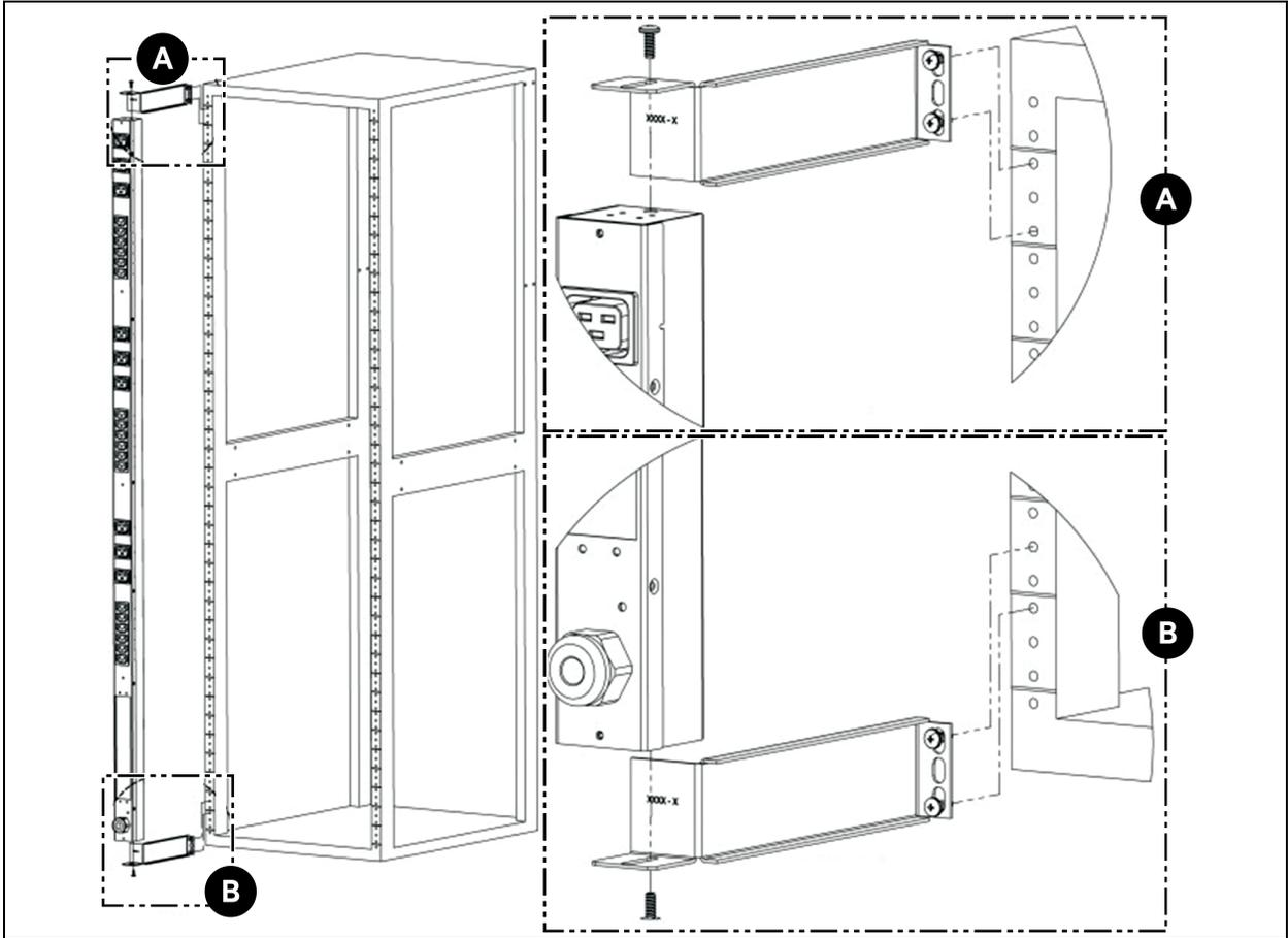
Figure 3.9 Flush Mount Bracket
